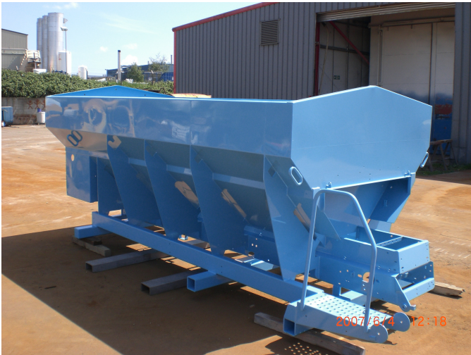
Above: A gritter body designed for salting the UK's roads. Blasted and zingaised and painted by Emtrade in Hull, UK.
