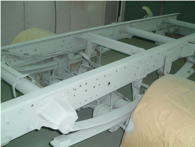
Above: The zingaised chassis of a cattle truck finished by McLarens of Irvine, Scotland
