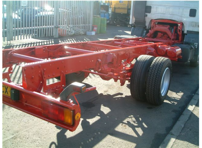
Above: The chassis with an automotive 2K polyurethane finish. Urine from the cattle damaged the old coating.
