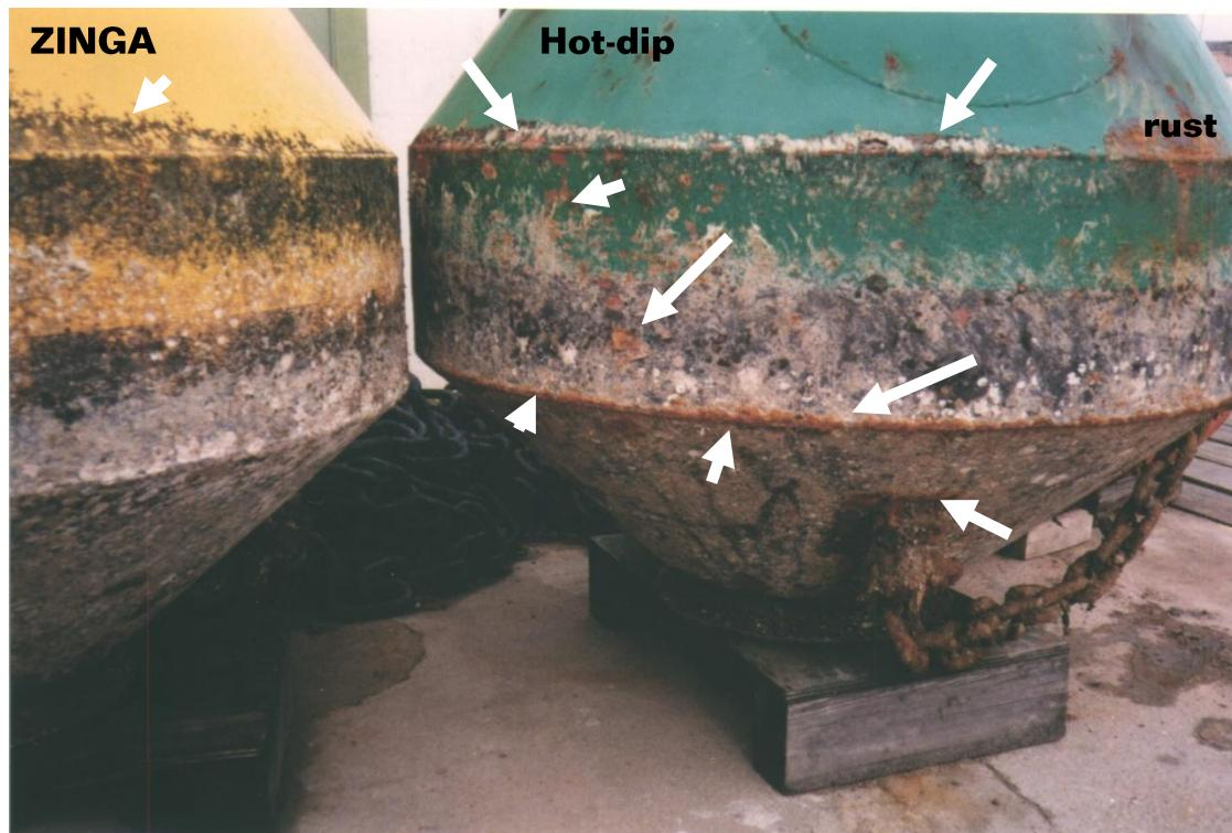
Conclusion of this test: the buoy treated with Zinga showed no trace of rust, but the hot-dip galvanised buoy was severely corroded in several places.
